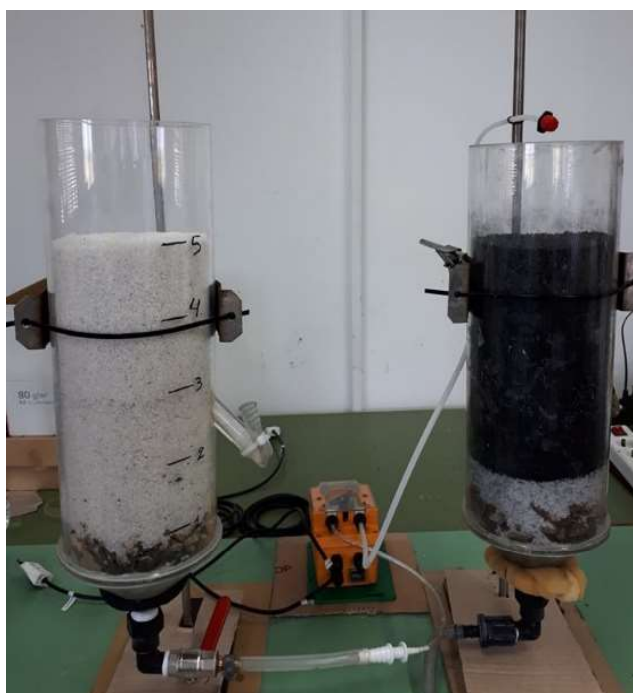
Figure 1. The installed laboratory-scale sand and activated carbon filter systems.
